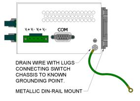
If the use of shielded cables is required, it is generally recommended to only connect the shield at one end to prevent ground loops and interfere with low level signals (i.e. thermocouples, RTD, etc.). Cat5e cables manufactured to EIA-568A or 568B specifications are required for use with N-Tron devices.
