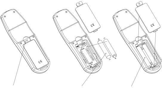
Press in and lift tab to remove battery cover out of recess.
