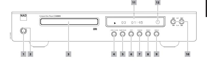
1 **STANDBY:** Press this button to switch ON the C 545BEE. The Standby LED indicator will turn from amber to blue and illuminate the Vacuum Fluorescent Display (VFD). Pressing the Standby button again turns the unit back to standby mode.
