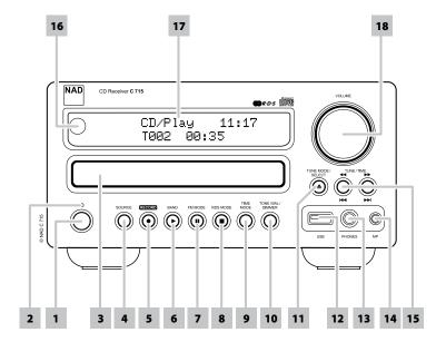
1 POWER: Press this button to switch ON the C 715. The Standby LED indicator will turn from amber to blue and illuminate the Vacuum Fluorescent Display (VFD). Pressing the power button again turns the unit back to standby mode.
