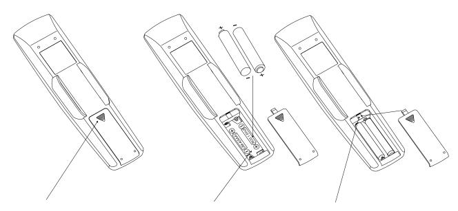
Press in and lift tab to remove battery cover out of recess.
