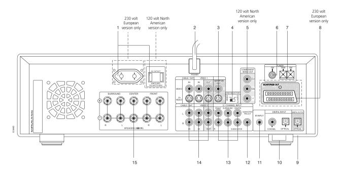
1 SWITCHED AC OUTLET: This convenience jack can supply switched power to another component or accessory. It is powered on and off by the front panel POWER key (or the HTR L70's ON and OFF keys).
