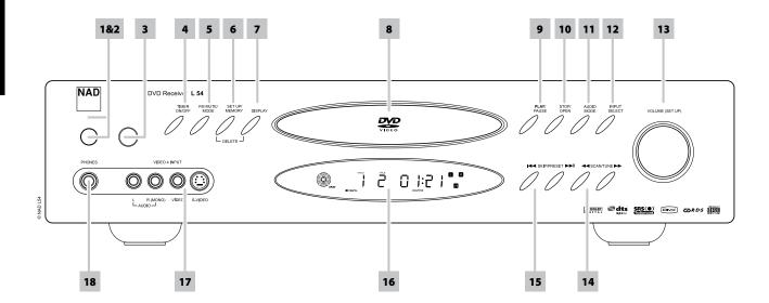
1 POWER: When the L 54 is first plugged into the AC power, the L 54's clock will light in the main Vacuum Fluorescent Display (VFD) display showing the time of day. Press to switch ON the L 54 from standby, changing the standby indicator from bright blue to dark and illuminating the VFD display. Pressing the power switch again turns the unit back to standby. It is usual (and perfectly acceptable) to leave the L 54 in standby mode in between normal viewing and listening sessions.
