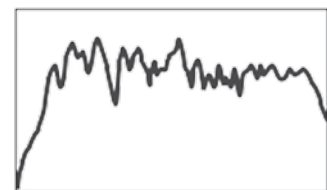
Inverse Correction Filter calculated by NAD T 175
