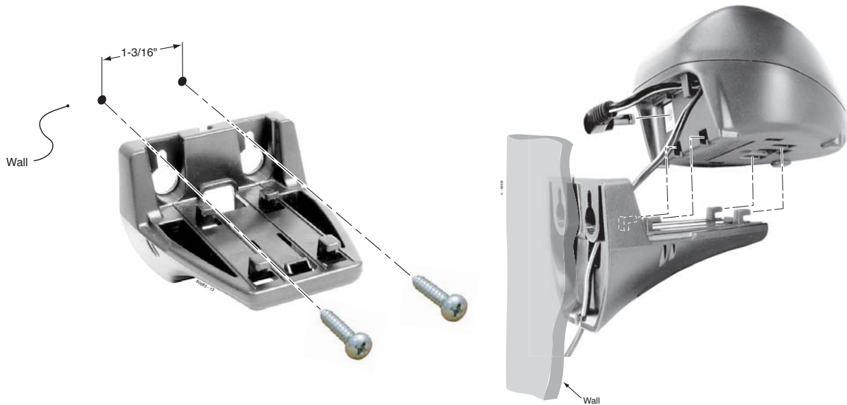
Figure 10: Wall-Mounting the Charger
