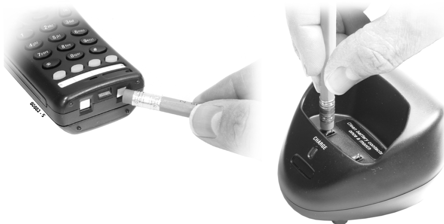
Figure 9: Cleaning the Battery Charger Contacts
