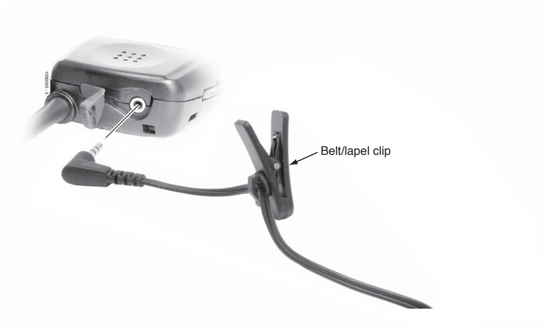
Figure 15: Connecting the Headset
