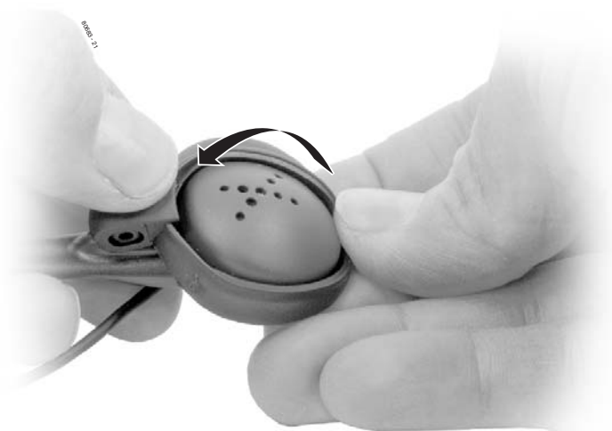
Figure 19: Snapping on the Earloop Ring
