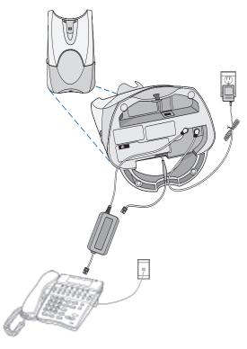
Connect the AC Power Adapter to the AC Power Adapter Jack on the underside of the Dterm Headset Cordless II Base. Plug the AC Power Adapter into the power source
