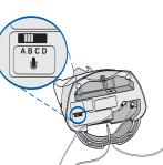
For NEC telephones, connect the Short Cord to the AP(R)-R adapter and then connect the AP(R)-R adapter to the telephone.
