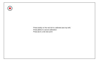
2. Press the center of the red dot with the stylus pen.
