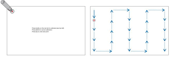
When all points indicated by the red dot are pressed by the stylus pen, calibration is completed and the calibration completion message is displayed on.
