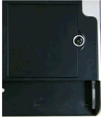
Fig. 3 Removing the memory cover
