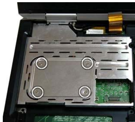
Fig. 17 Removing the heat plate screws
