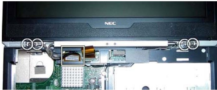
Fig. 21 Removing LCD connector and hinge screws
