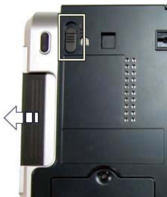
Fig. 2 Removing the Versa Bay IV Module
