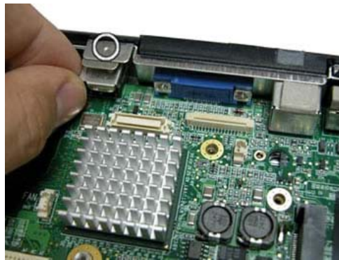
Fig. 31 Removing the AC socket holder
