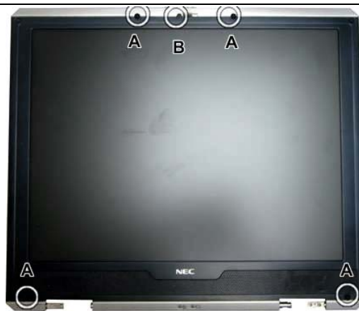
Fig. 22 Removing rubbers and screws
