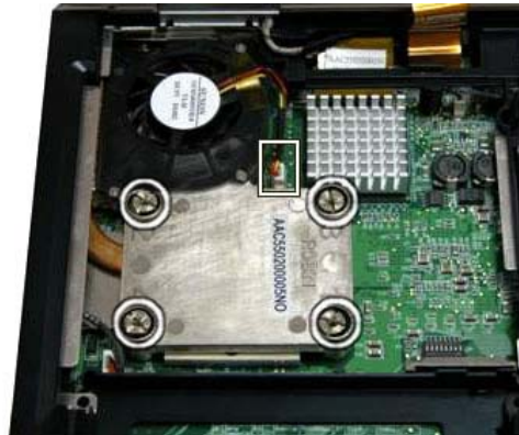
Fig. 18 Removing the heat sink screws and fan connector
