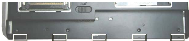
Fig. 29 Disengaging the latches in the battery compartment
