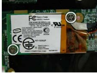
Fig. 33 Removing the MDC modem
