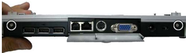
Fig. 28 Removing screws on the back of the system
