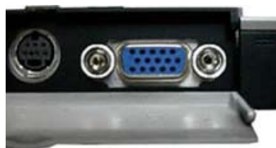
Fig. 32 Removing VGA port screws
