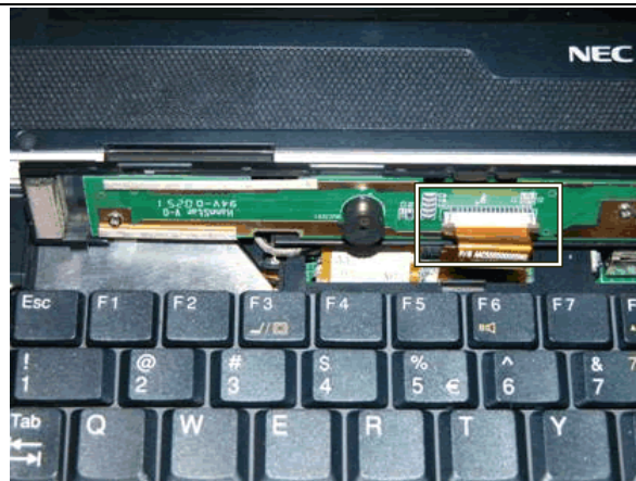
Fig. 7 Disconnecting the keyboard cover cable
