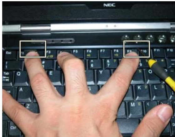
Fig. 6 Removing the keyboard cover
