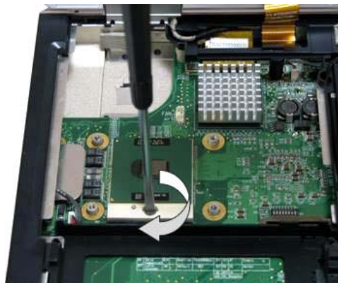
Fig. 19 Releasing the CPU lock
