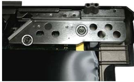
Fig. 30 Removing the Versa Bay shield
