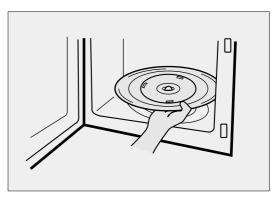
7 The roller guide and oven cavity floor should be cleaned regularly to avoid excessive noise.
