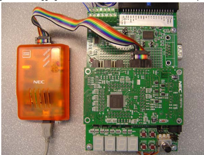
Figure 11. Debugging Environment Shown with QB-78K0MINI On-Chip Debugger
