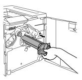
${f 3}$  Support the bottom of the drum with your hand, then carefully pull the cartridge toward you and remove it.
