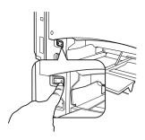
2 Remove the cover from the right side of the printer. Use a Phillips screwdriver to remove the two screws securing the right cover.
