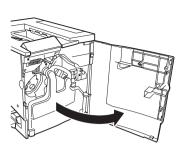
6 Remove the protective cover clearly marked "Remove."
