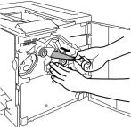
6 Rotate the transfer belt release lever counterclockwise to its correct position (7 o'clock).
