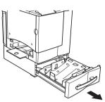
Make sure that the paper fits easily between the guides and the paper corners are under the left and right mediaseparating tabs and are not bent.
