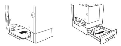
When refilling media, first remove any media remaining in the tray. Stack it with the new media, even the edges, then reload it.
