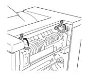
When removing the jammed media, be careful not to touch the transfer belt. Touching the transfer belt may result in decreased print quality.
