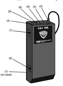
volume is too low, turn the OUTPUT LEVEL CONTROL (7) clockwise until you obtain comfortable volume.
