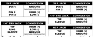
Paralleling inputs and outputs may be accomplished by using any of the 3 connectors. *Note: The 1/4" TRS are normally used for this*
