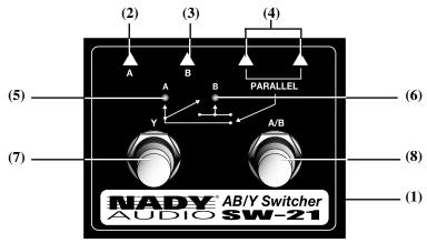
(1) 9VDC Battery Compartment — Battery only functions to power LED indicators and unit can operate without the LEDs. Change battery when LEDs become dim.
