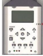
ARES-P: Has no USB connector. The card is formatted "Linear File" non-compatible directly with Windows except if the Ares Import software is used. The recorded files can be G.722 or MPEG 1 layer II. Maximum bitrate is 192kb/s 48kHz stereo (96kb/s per channel).
