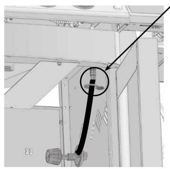
Ensure the regulator drops into the small opening, between the tank heat shield and the right side of the cabinet.
