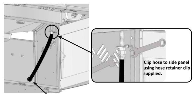
Install bushing into rear panel.
