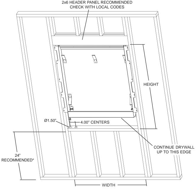
CHECK WITH YOUR LOCAL BUILDING AUTHORITY FOR COMPLETE FRAMING GUIDELINES. THE CHART BELOW WILL GIVE YOU THE OPENING SIZE REQUIRED FOR EACH MODEL. EACH WATERFALL IS INTENDED TO BE MOUNTED ON TOP OF THE DRYWALL (NOT SHOWN). THE DRYWALL BELOW THE UNIT SHOULD CONTINUE UP TO THE BOTTOM OF THE WATERFALL BASIN.
