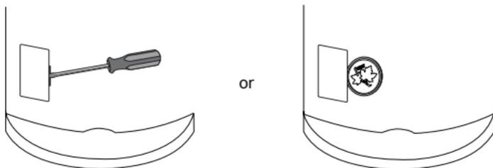
2. Replace the battery with a new SR44, with the + side facing up.
