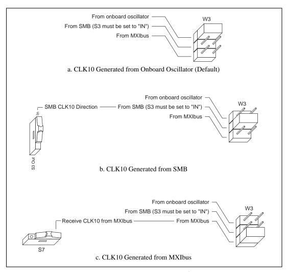
Figure 3-5. VXIbus CLK10 Routing
