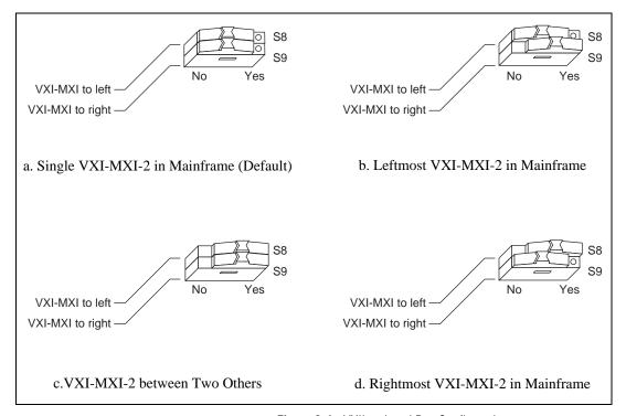
Figure 3-4. VXIbus Local Bus Configuration
