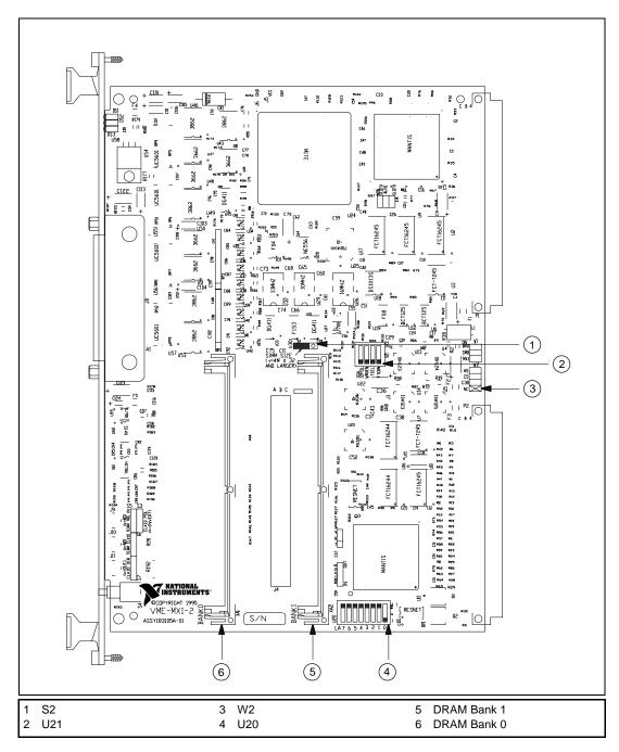
Figure 4-1. VME-MXI-2 Parts Locator Diagram
