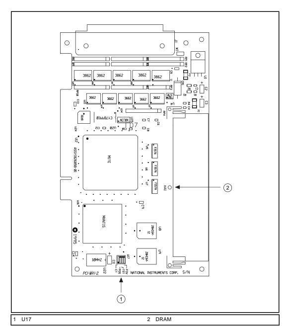
Figure 2-1. PCI-MXI-2 Parts Locator Diagram
