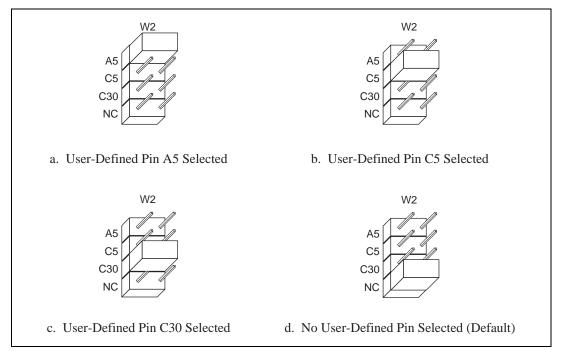
Figure 4-3. VME-MXI-2 Intermodule Signaling Settings
