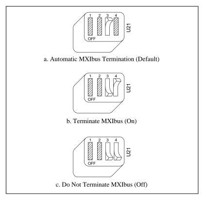
Figure 4-4. MXIbus Termination
