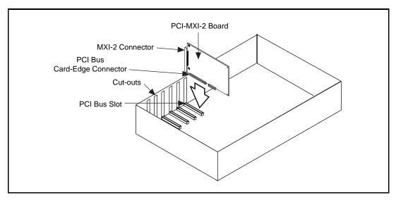
Figure 2-2. PCI-MXI-2 Installed in a Computer
