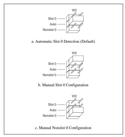
Figure 3-3. VXIbus Slot Configuration
