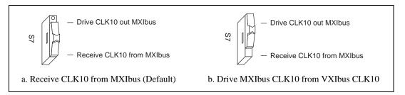
Figure 3-7. Receiving or Driving MXIbus CLK10
