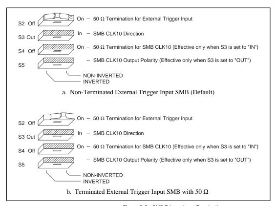
**Figure 3-8.** SMB Trigger Input Termination
