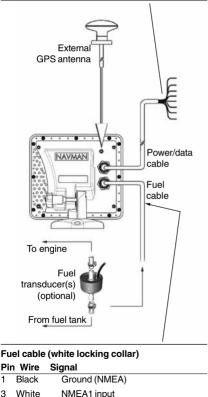
Note: Shield is connected to pin 1. black wire
