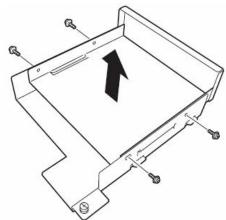
**5.** Fix the device to the tray for adding devices with the four screws.
