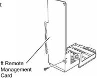
Check the slot for ft Remote Management Card and remove the connector cap installed in the slot.
