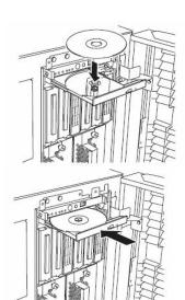
To remove the CD-ROM, press the CD-tray-eject button as you did in setting the CD-ROM.
