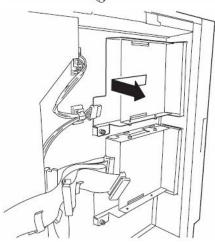
**4.** Remove the four screws securing the dummy cover, and remove the dummy cover.
