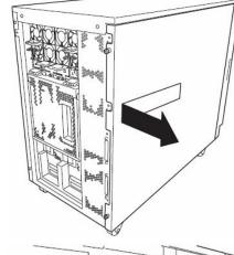
**3.** Loosen screws to remove the tray for adding devices.
