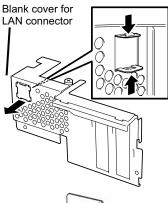
**4.** Install ft Remote Management Card to PCI rear bracket with one screw.
