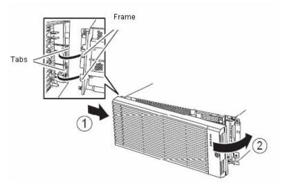
To attach the front bezel, engage the tabs on the frame on the left side of the main unit. After attaching and closing the front bezel, lock it with the key for security.
