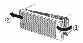
3. Detach the front bezel from the main unit by sliding it to the left a little to disengage the tabs from the frame.
