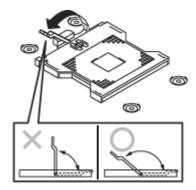
**8.** Place the CPU on the socket carefully.
