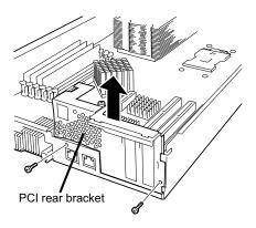
**3.** Remove the blank cover for LAN connector of ft Remote Management Card. Grab the top and bottom of the blank cover to unlock and remove it.
