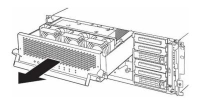
**6.** Carefully place the CPU/IO module on a flat and sturdy table.
