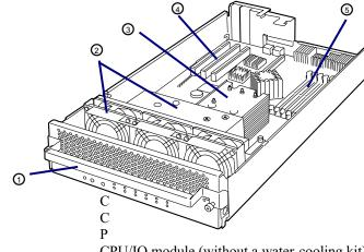
CPU/IO module (without a water-cooling kit) (320Fa-L/320FaLR model)
