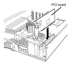
**6.** Insert the board for connecting part of the board to securely connect to the slot.
