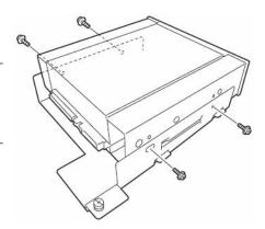
Gently insert the device into the tray and secure it with the screw.
