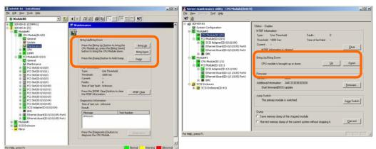
**NEC ESMPRO Manager** Select [ft] - [CPU Module] - [CPU Module (to be removed)] - [Maintenance] - [Bring Up/Bring Down] - [Bring Down].
