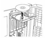
Press the locking part in the center of the tray and pick the CD-ROM gently. When you have removed the CD-ROM, push the tray to the drive-closed position.
