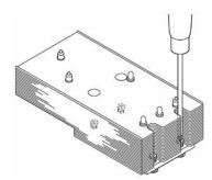
**13.** Confirm that the heat sink is mounted horizontally to the motherboard.
