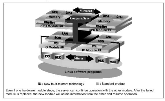
NEC Express5800/ft series is a highly fault-tolerant server that achieves continuous computing operations, data storage mirror, and continuous network connection. It allows you to run Linux-based applications.
