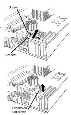
**4.** Remove the connector cap installed in the slot in which the board is installed.
