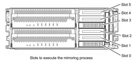
Empty slots in the 3.5-inch hard disk drive bay contain dummy trays. The dummy trays are inserted to improve the cooling effect within the device. Always insert the dummy trays in the slots in which hard disks are not installed.
