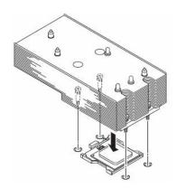
**12.** Secure the heat skink with the screws. Firstly, fasten four screws in a crisscross pattern tentatively, then fasten the screws tightly.
