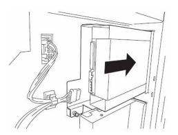
7. Connect the SCSI cable and power cords to the device.
