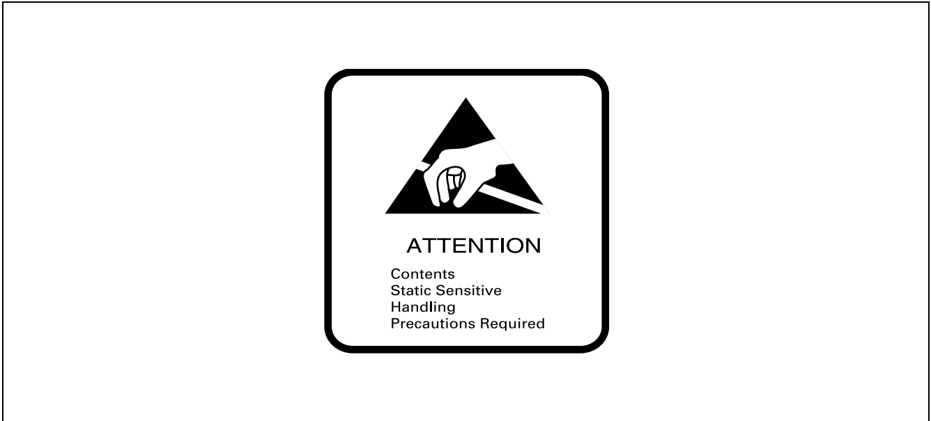
Figure 4-2 Static Caution Indication
