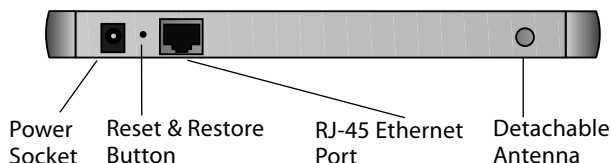
Figure 2-2: WG602v3 rear panel
