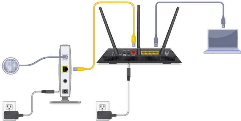
Figure 7. Modem router cabling for cable or fiber service
