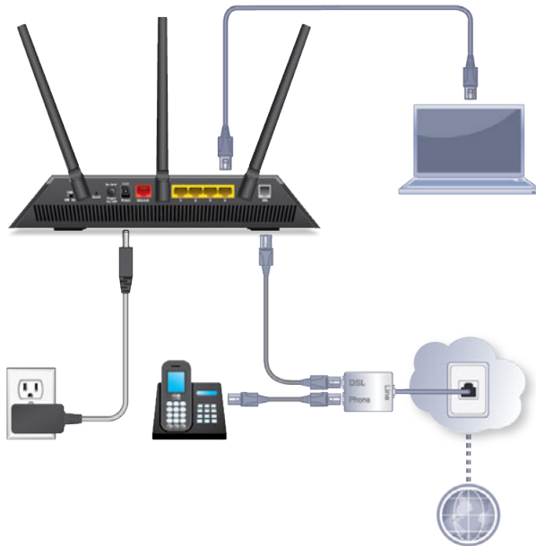
Figure 6. Modem router cabling for DSL service
