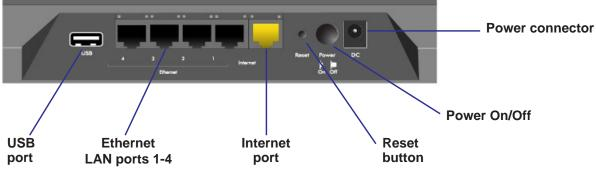
Figure 3. Router, rear view
