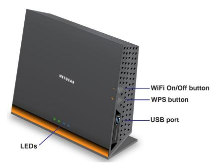
Figure 2. Router, front and side view
