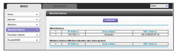
Wired devices are connected to the router with Ethernet cables. Wireless devices have joined the wireless network.
