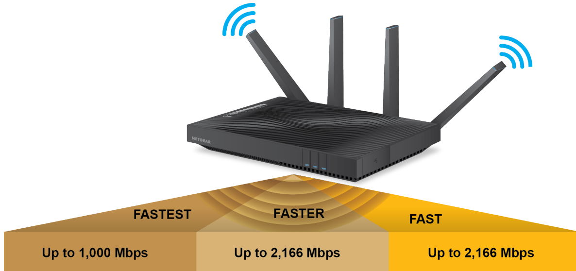
Figure 6. Tri-band WiFi doubles the available bandwidth for dual-band devices
