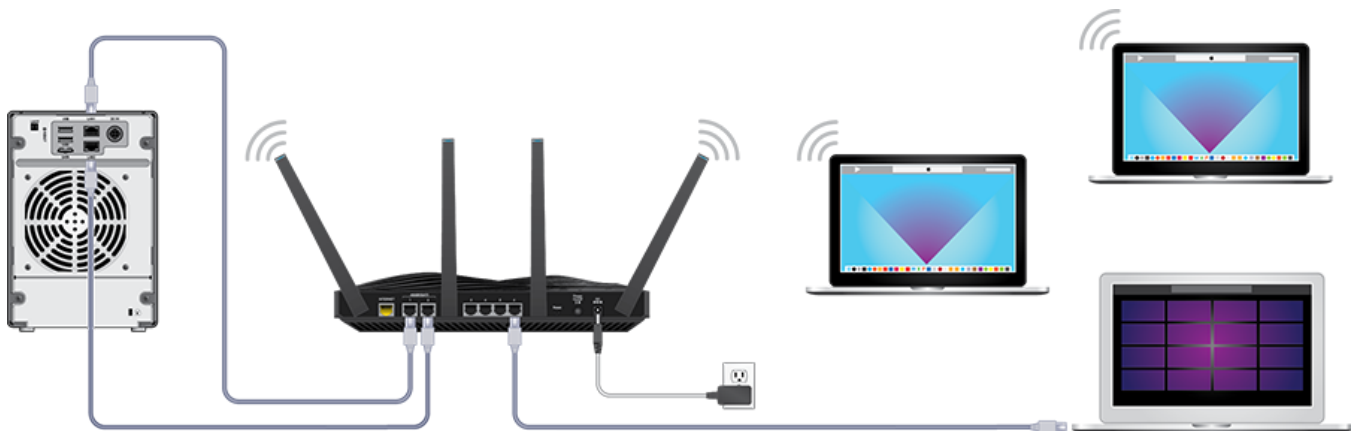
Figure 11. Ethernet port aggregation
