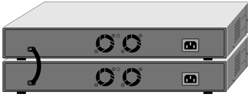
Figure 4-3. Cabling Two FS517TS Stacked Switches
