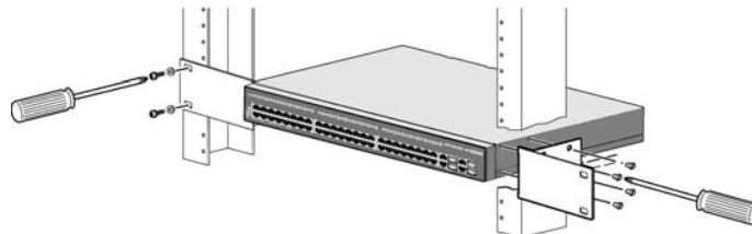
Figure 3-1. Attaching Mounting Brackets
