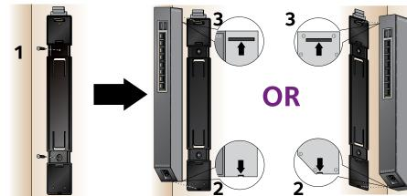
Note: You must screw the backplate into a wall stud when wall mounting the switch.
