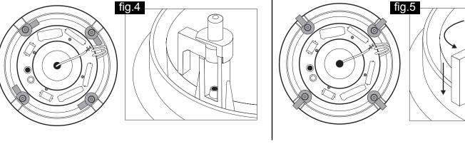
**6.** The bezel (with driver) attaches to the bracket via four plastic mounting clamps on the back of the bezel that swivel to "sandwich" the drywall between the bezel frame and the clamps (fig.4). First rotate the mounting clamps counterclockwise so that the body of the bezel can slide through the mounting bracket. Exercise caution not to damage the driver.
