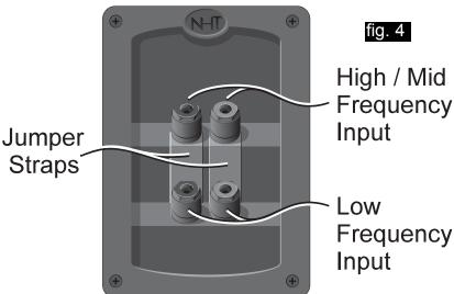
speakers. Prepare your speaker wire by stripping 1/4" to 3/8" of insulation from the ends and twisting the exposed wire strands tightly. The five-way binding posts on the back of the speaker will accept raw wire, banana plugs, or spade plugs. Tighten the binding posts by hand, as pliers can strip or break them.
