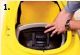
Grab the bottom edge of the backrest and tilt it back to at least 45 degrees to the strut that holds it up.
