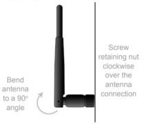
Note: Do not over-tighten the attaching nut - but do make sure that
