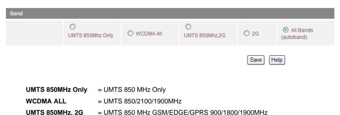
= GSM/EDGE/GPRS 900/1800/1900MHz All Bands (autoband) = UMTS 850/2100/1900MHz GSM/EDGE/GPRS 900/1800/1900MHz
