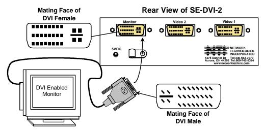
3. Connect the video sources to their corresponding DVI ports labeled "VIDEO 1" and/or "VIDEO 2" on the rear panel of the VIDMUX using male-to-male DVI-I cables.
