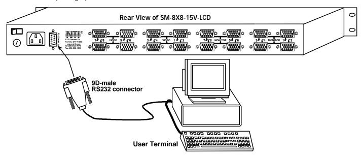
Figure 3- Connect user terminal for RS232 control
