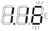
With the desired port number selected, point the IRT at the switch/receiver and press the "OUT" button to transmit the selection and make the change. The blinking number in the LCD will stop blinking. An LED on the receiver will illuminate.
