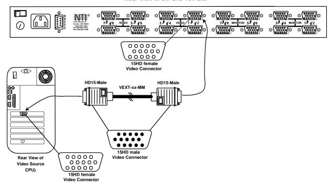
Figure 1- Install Video Source Cables
