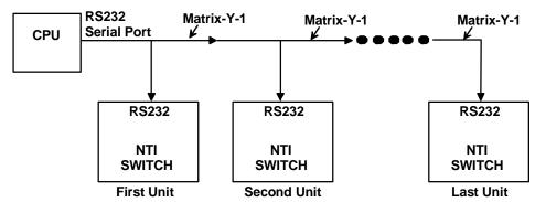
Figure 6- RS232 connection with Matrix-Y-1 cable
