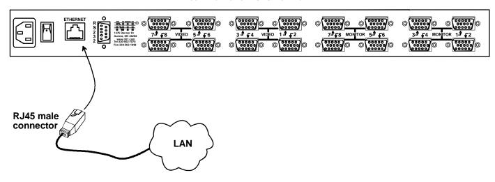
Figure 4- Connect the LAN to the VEEMUX
