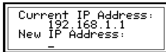
Figure 16- Set IP Address from LCD and keypad
