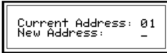
Figure 14- Set Serial Address from LCD and keypad
