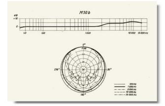
frequency response to above 1000 Hz with a gradual rise reaching +6 dB from 8000 to 16000 Hz. Simultaneously, the directional characteristic shows an increasing directiv-
