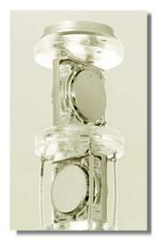
al, cardioid, or figure-8. In a stereo microphone two capsules of this type are mounted one above the other in a single head. Combined with two microphone amplifiers, placed alongside one another in a tube measuring only 30 mm in diameter, the SM 2 was created.
