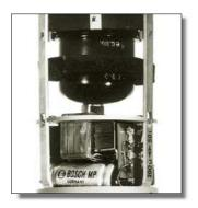
perforations in the electrode. The sound also reaches the outside of the rear membrane. The acoustic properties of the center electrode cause the forces acting on the rear membrane to be equal in size, but opposite in direction. Therefor, the rear membrane does not move and does not produce any electrical signal. For sound arriving from behind, the rear membrane moves and the front membrane does not. As a consequence, the microphone does not re-
