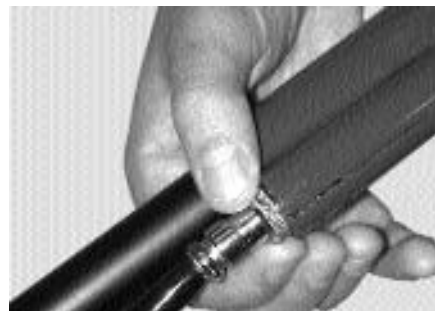
Figure 11. Hand-tighten the locking nut
