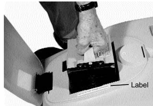
Figure 13. Orient and insert the battery
