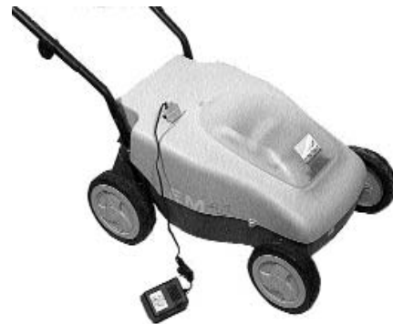
Figure 22. Charging the battery in the Mower
