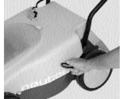
Figure 18. Cutting height lever set to leave your grass 1.6 inches high
