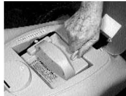
Figure 3. Turn the battery retainer arm
