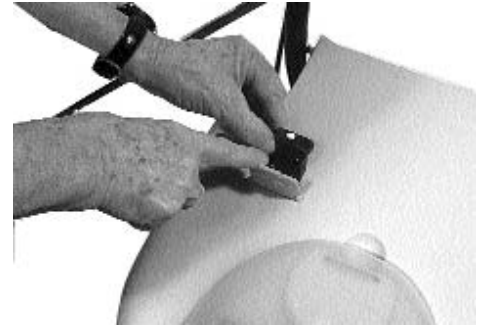
Figure 19. Insert the safety key
