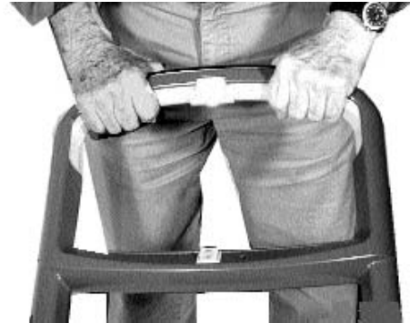
Figure 21. Squeeze the orange control bar
