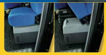
**Instructor seat and removable cool box** All models are fitted with a well upholstered instructor seat. For additional comfort, when Automatic Temperature Control (ATC) is fitted, a purpose-designed cool box is included. The latter operates from both 12V and mains power.
