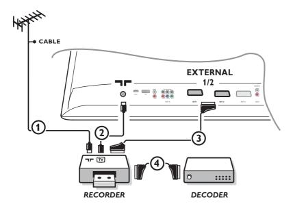
Note: Do not place your recorder too close to the screen as some recorders may be susceptible for signals from the display. Keep a minimum distance of 0.5 m from the screen.
