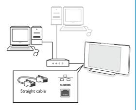
Push the other end into a free Ethernet connector on your router.
