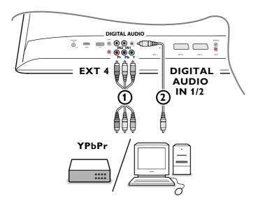
• Connect the three separate component video cables (1) to the peripheral equipment having component video outputs (YPbPr), such as DVD-players, laser-disc players, videogame players, satellite receivers or other equipment, and to the **Y**, **Pb** and **Pr** jacks of **EXT4** on the TV.
