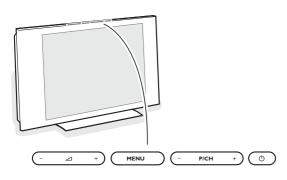
Should your remote be lost or broken you can still change some of the basic settings with the keys on the top of your TV. Press the power switch  $\binom{1}{2}$  to switch the TV on.
