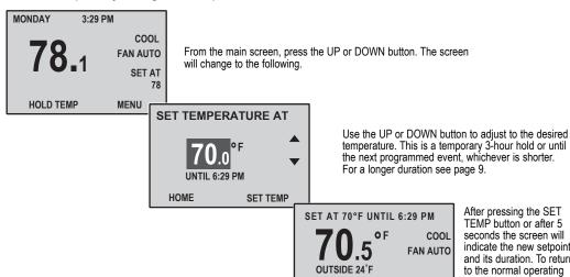
After pressing the SET TEMP button or after 5 seconds the screen will indicate the new setpoint and its duration. To return to the normal operating program mode, press RESUME PROGRAM
