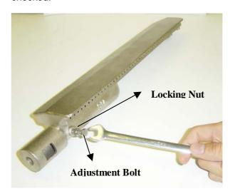
Flames should be blue and stable with no yellow tips, excessive noise or lifting. If any of these conditions exist, check to see if the air shutter or burner ports are blocked by dirt, debris, spider webs, etc. If you have any questions regarding flame stability, please call customer service at 1-800-913-8999.
