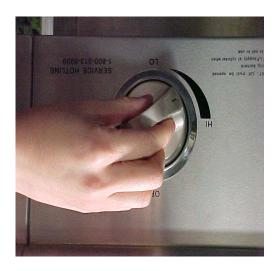
Step 3. You may need 3 or 4 trials to light the burner. After the burner is lit, adjust the knob as desired
