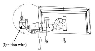
Step 2: Remove 4(four) screws & washers from the "U" brackets on the side burner
