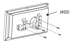
Step 4: Insert valve stem assembly through knob hole to the control panel
