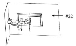
Step 7; Tight all 4(four) screws on the "U" brackets on the burner, then connect the ignition wire on to valve.
