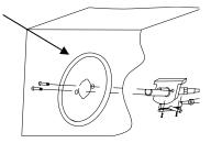
Step 8: Place knob on valve stem, then screw the knob by using the wrench tool.
