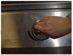
Step 2. Push and turn one of main or side burner knobs to HI position
