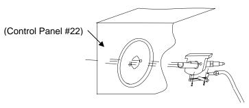
Step 6: Align & tighten knob bezel & valve stem with 2(two) screws & washers as shown below. (knob bezel in bag)
