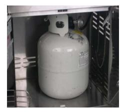
□ Secure the gas tank by turning the retention screw at the right of the grill clockwise until it is tight.
