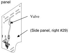
Step 3: Insert valve stem assembly into burner venturi
