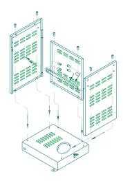
**Step 3**: Assemble the head part to the bobywork part. Remove the head unit of grill from carton. Insert the upper portion of the grill onto the cart from the top with four (4)1/4\*13mm screws. **Caution!! The firebox is heavy, and we recommend two or more people to lift up firebox.**
