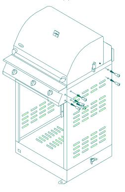
**Step 6 :** Assemble the fortified steel to the main with (8)1/4'\*13.
