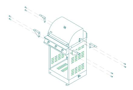
Step7: Assemble side shelf and side burner with four(8) 1/4\*13mm screws as figure show below .
